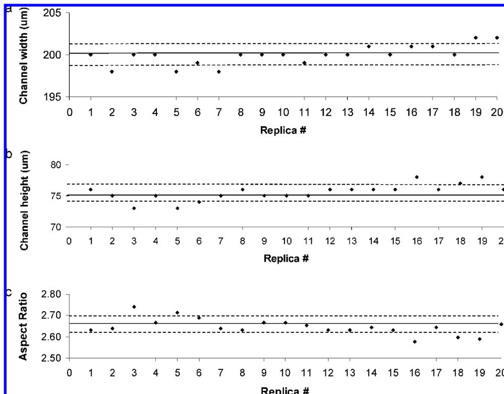
**Figure 7.** Comparison of the channel width (a), height (b), and the aspect ratio (c) of the 20 PMMA embossed replicas. The solid line represents the mean, and the dotted lines represent  $\pm 1$  standard deviation of the mean.
