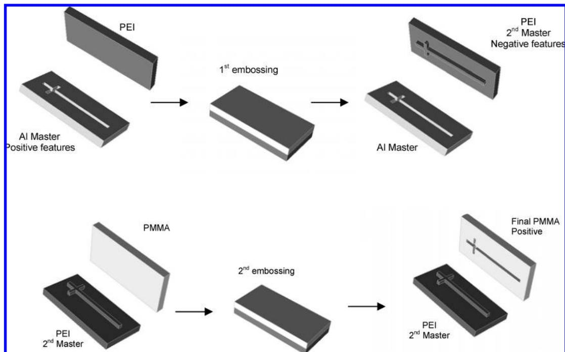
**Figure 2.** The two-stage embossing process, from primary aluminum master to final PMMA chip. The aluminum master serves as the primary mold in the embossing process. In the first embossing step, the positive features of the aluminum master are imprinted as negative features into a PEI substrate to produce the secondary mold. In the second embossing step, the negative features of the secondary mold are imprinted as positive features into a PMMA substrate to produce the final chip.
