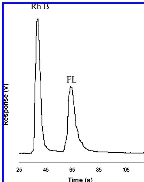
**Figure 9.** Electropherograms showing an on-chip electrophoretic separation of a  $10^{-3}$  M RhB/ $10^{-3}$  M FL test mixture.
