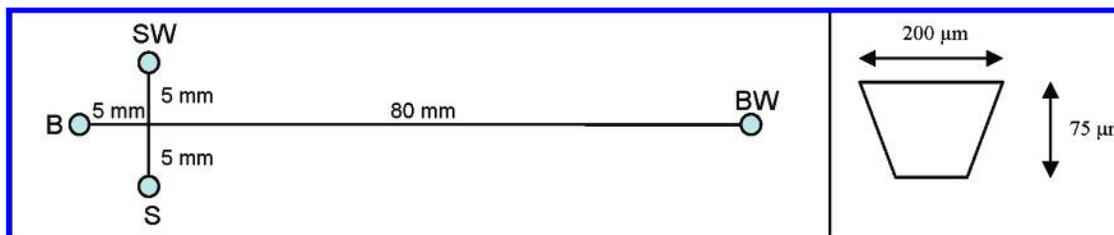
**Figure 4.** Schematic of the microchip layout showing the channel lengths and the approximate cross-sectional dimensions. Each channel has a 1.5-mm-diameter well at each end; the wells are labeled buffer reservoir (B), buffer waste (BW), sample reservoir (S), and sample waste (SW).
