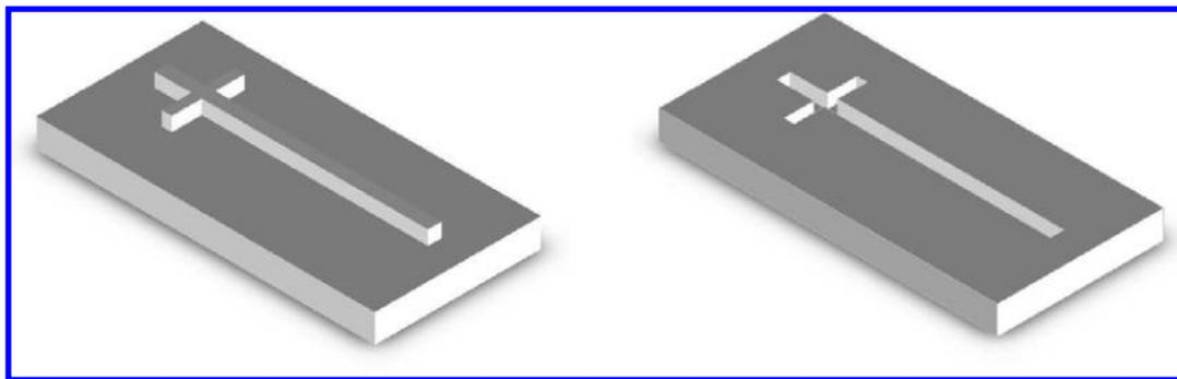
**Figure 1.** Master designs produced by micromachining. Recessed features (right) created by cutting into the metal stock and raised features (left) created by removing the excess metal around the desired feature areas result in molds to be used for feature replication.
