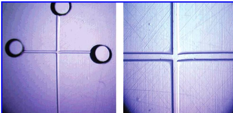
**Figure 5.** A cruciform PMMA microchip at 6× (left) and 40× (right) magnification.
