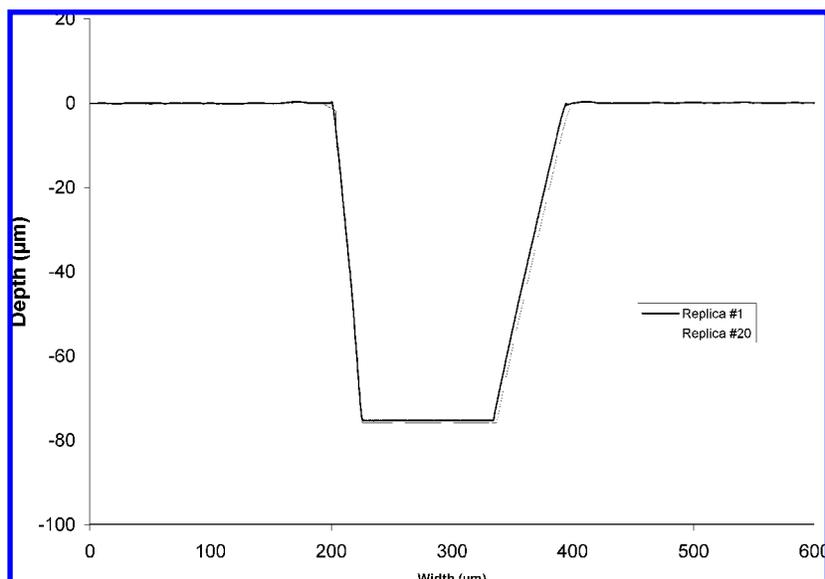
**Figure 6.** Measurements of the microchannel features obtained by surface profilometry. Depths and widths of the main channel in PMMA replica no. 1 (solid line) vs PMMA replica no. 20 (broken line) are compared.
