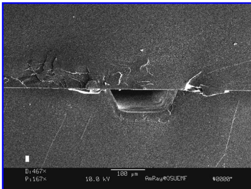
**Figure 8.** SEM image of a PMMA microchip showing the channel cross section. For imaging, the chip was frozen in liquid nitrogen and fractured to provide a cross section for imaging.
