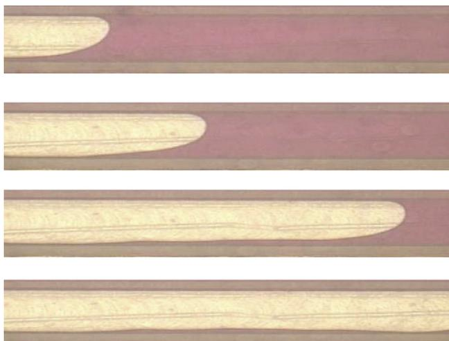
Fig. 7. The channel was formed by conformally sealing the APET chip with a PDMS slab, and filled with  $10^{-3}$ M Rhodamine B dye in methanol under a very low pressure.
