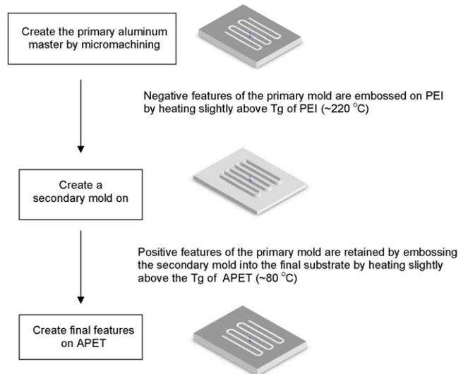
Fig. 3. Schematic diagram of the two-stage embossing procedure.
