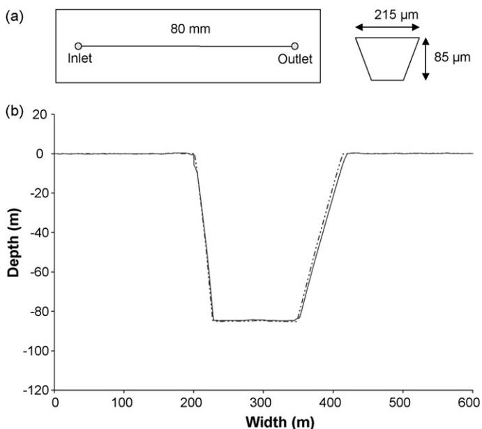
Fig. 4. (a) Schematic of the microchip layout showing the channel lengths and the approximate cross-sectional dimensions. (b) Measurements of the microchannel features obtained by surface profilometry. Depths and widths of the channel of the primary aluminum mold (--- line) vs. APET replica #8 (solid line) are compared.
