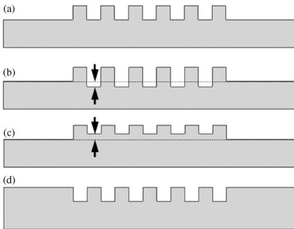
Fig. 2. An illustration of the impact of micromachining tool-offset error (black arrows) on the co-planarity of macroscale and microscale features; (a) co-planar with no tool-offset error; (b) excessive tool-offset; (c) insufficient tool-offset and (d) tool-offset independent.
