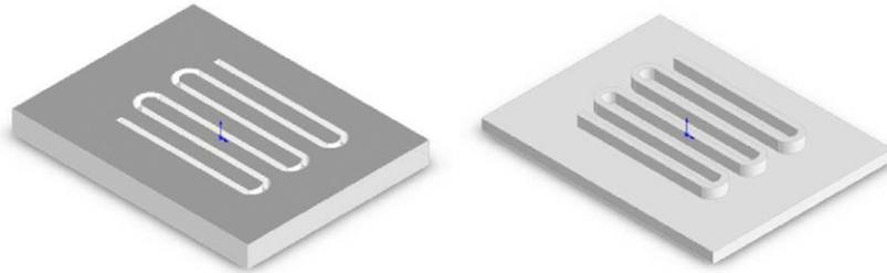
Fig. 1. Master designs produced by micromachining. Recessed features (left) created by cutting into the metal stock, and raised features (right) created by removing the excess metal around the desired feature areas, result in molds to be used for feature replication.
