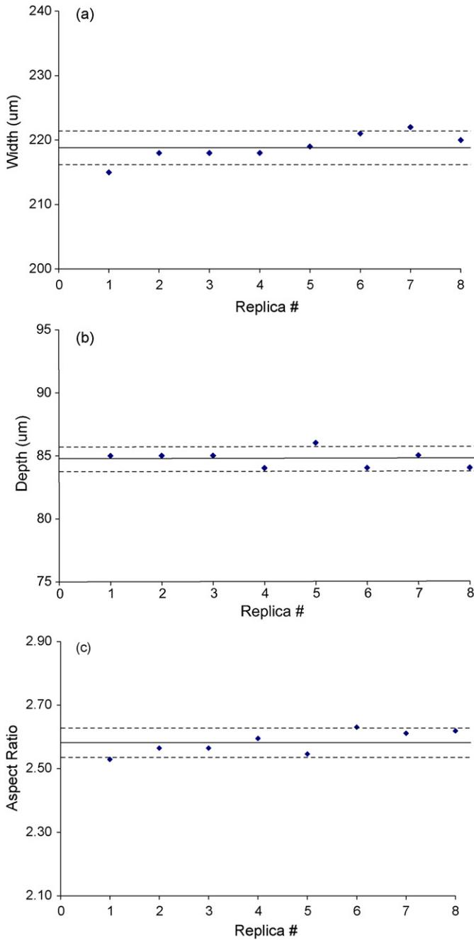
Fig. 5. Comparison of the channel width (a), depth (b), and the aspect ratio (c) of the 8 APET embossed replica. The solid line represents the mean, and the dotted lines represent  $\pm 1$  standard deviation of the mean.
