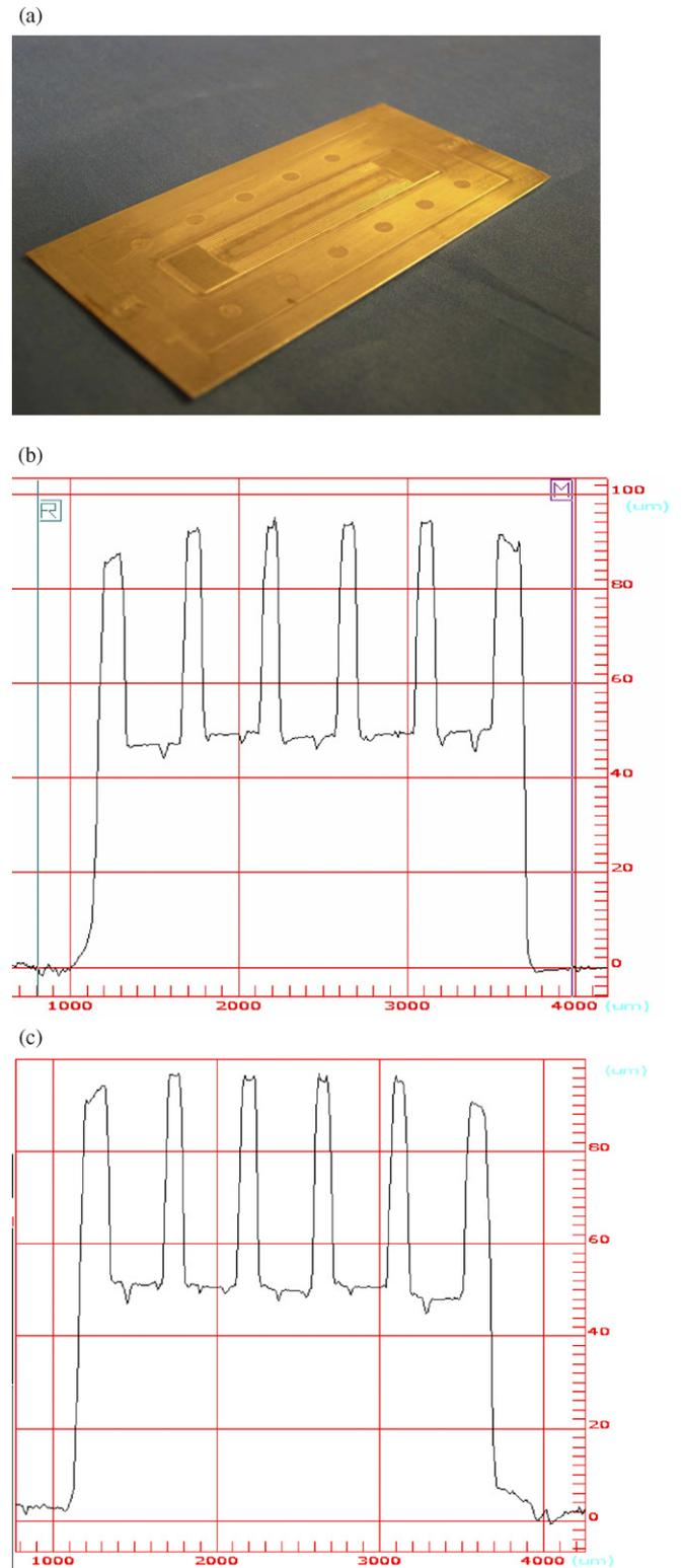
Fig. 6. Photograph of the aluminum primary mold (a), surface profile of primary mold (b) and APET substrate (c) measured with the profilometer.
